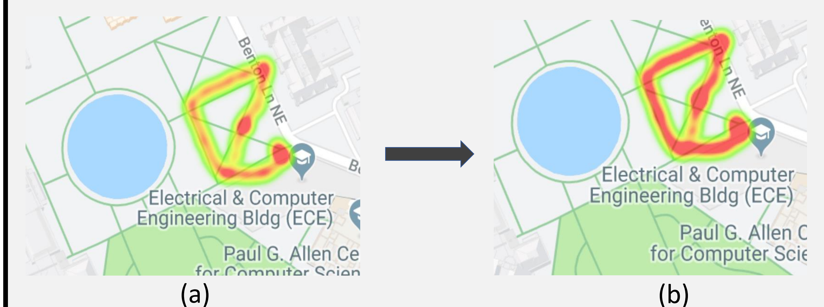
Figure 3. (a) Trajectory using GPS sensor data (b) Trajectory based on Kalman filter using IMU data and few GPS sensor data
