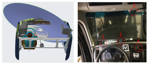
Figure 2: (left) CAD model with mannequin, eyepoints, and camera FOV. Figure 3: (right) Final locations of the 4 cameras used for testing.
